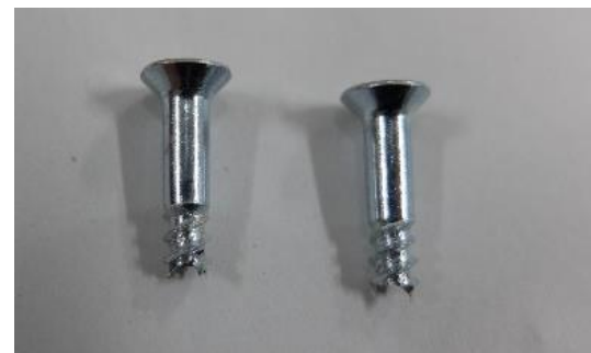
Fracture of fastener (4.1×38mm)
