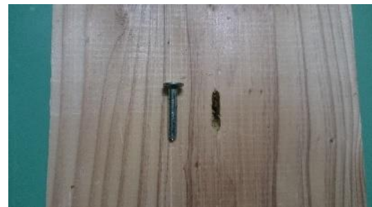
Fracture of fastener (CN50)
