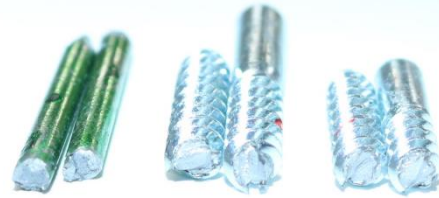
Fig. 3.4 Fracture behavior of constant-amplitude reversed cyclic bending test for fasteners
