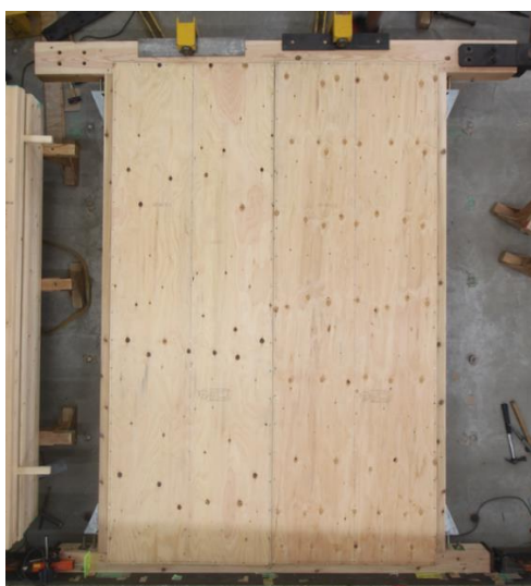
Fig. 5.2 State of specimen installation (shear wall test)
