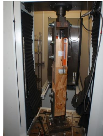
Fig. 4.2 State of specimen installation in the single shear test of joint
