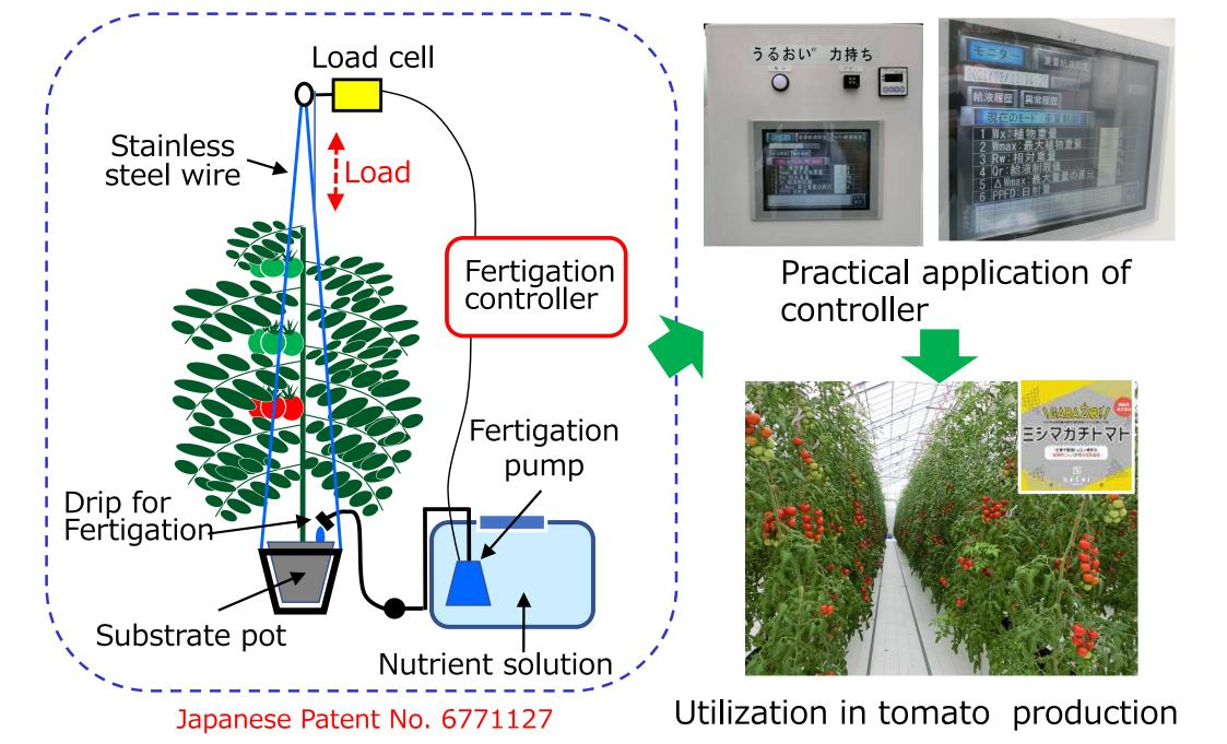
Development of a fertigation Control System Using Load Cells for High-Sugar & High-functionality Tomato Hydroponics
