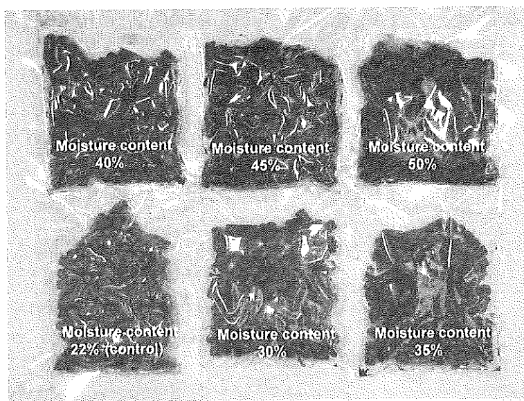
Fig. 2 Appearance condition of enclosed and conserved pellets by nylon poly-bag (30°C, 3 months)
